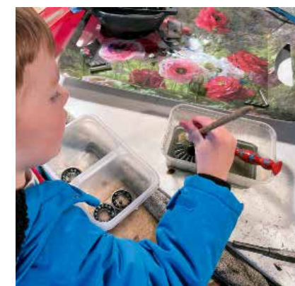
ABOVE Matthew cleaning the cogs; worn ball bearing to the right of less worn bearing
