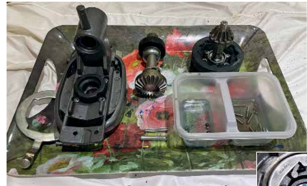
LEFT Use a tray when deconstructing the gearbox to keep all of the components together INSET BELOW Needle roller bearings are held in place with grease during reassembly. The pawls will need to be oiled BELOW A messy, greasy business, but it's all coming back together nicely
